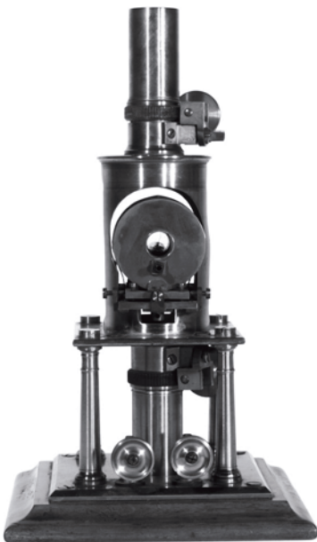
Fig. 9.1. Kelvin's cable galvanometer as used on-board the US Niagara . (Courtesy of the Photographic Library, Hunterian Museum and Art Gallery, University of Glasgow.)
