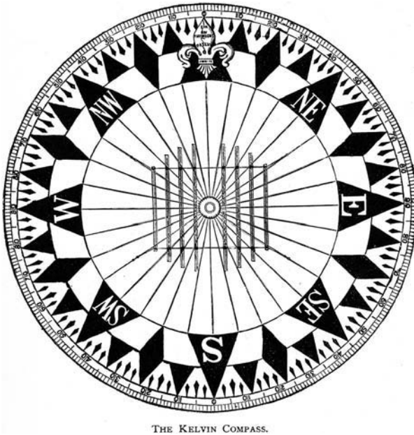
Fig. 9.6. Kelvin's compass card showing the eight magnets slung under the card and disposed symmetrically about the North/South axis (From Silvanus P. Thompson, The Life of William Thomson Baron Kelvin of Largs , 2 volumes, Macmillan & Co., London, 1910, p. 715.)
